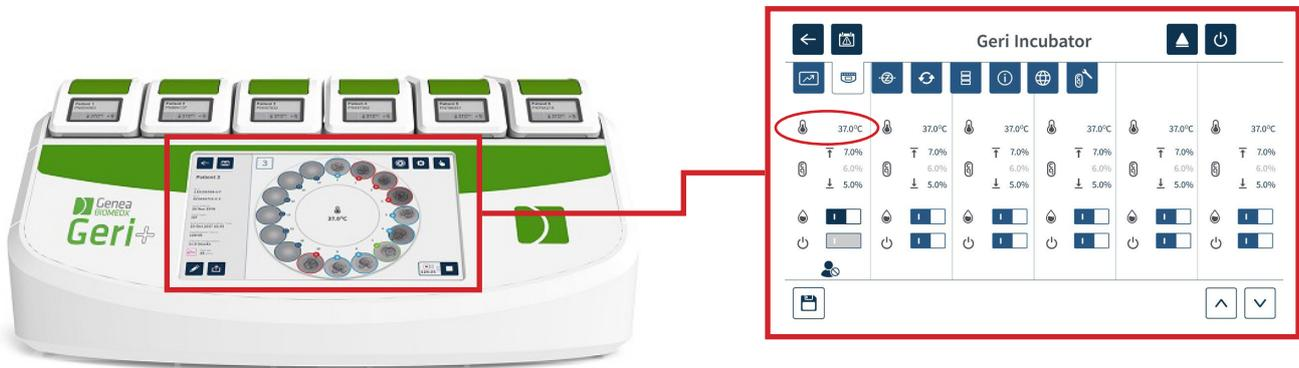
**STEP 2** Place **LEO's temperature probe (T1-MODULE)** inside the **Geri Dish**, as indicated in the following schematic. You can use two T1-MODULEs together to measure 2 chambers.
