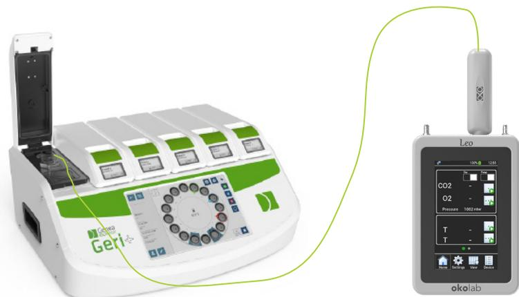
**STEP 3** Fill the dish with media and oil. Place the cable of **LEO's** probe so that the tip of the sensor touches the bottom of the central microwell dish, at the position where the embryos sit, and put the dish lid.
